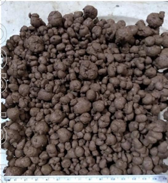
*Figure 1: A sample of the agglomerates showing samples are relatively uniform in size and shape, with good retention of fine material on coarser grains. They remained moist after curing but with negligible retention of excess moisture. A soak test determined that the agglomerates were stable in aqueous environments.*
